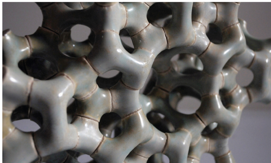
Figure 5: Slip cast, celadon glazed and fired structural members cast from 3D printed originals (top). Modular structure assembled from individual stoneware pieces (middle). Modular structure assembled from individual stoneware pieces (bottom).
